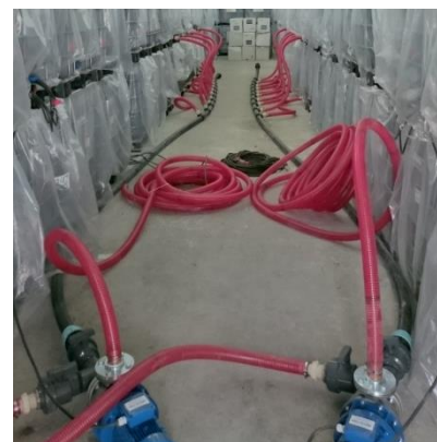
Figure 21 Dispersants loading system
